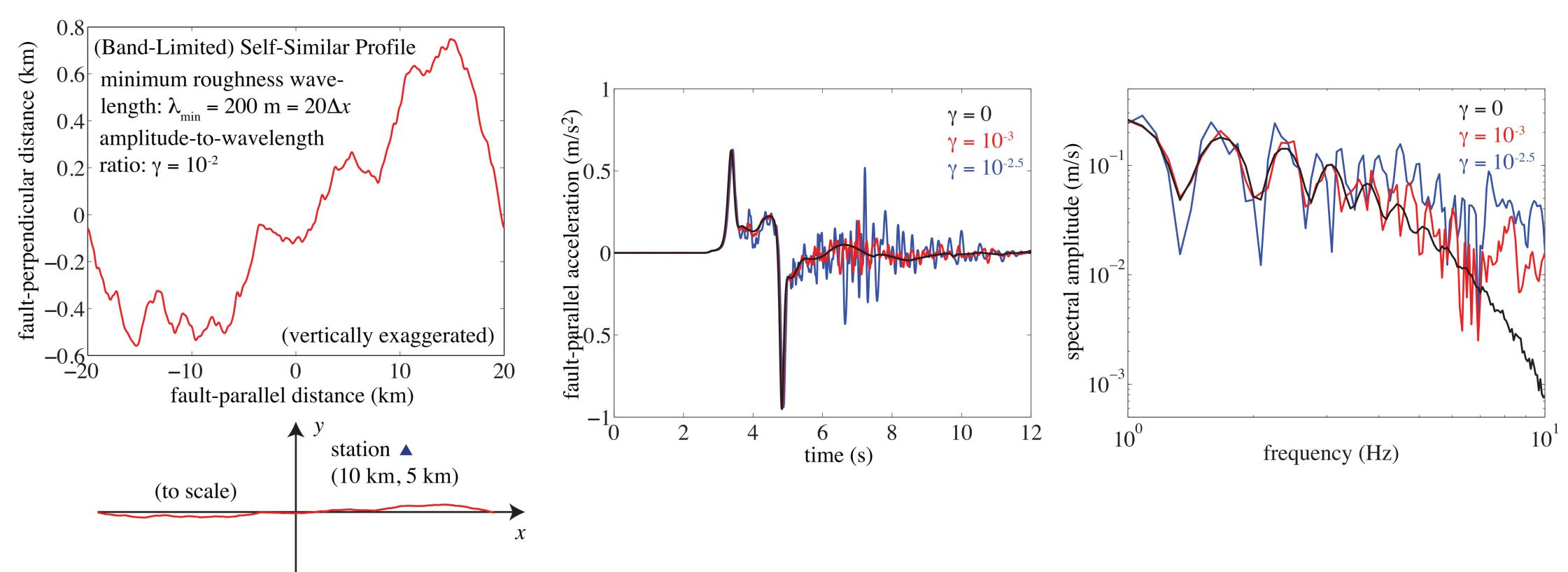
We modeled plane strain ruptures on rough faults with rate-andstate friction featuring strong dynamic weakening. (above), (below), and (right) Results from band-limited self-similar profile. Note large changes in normal and shear stress on fault. Changes will be even more extreme when shorter wavelength roughness is modeled.
