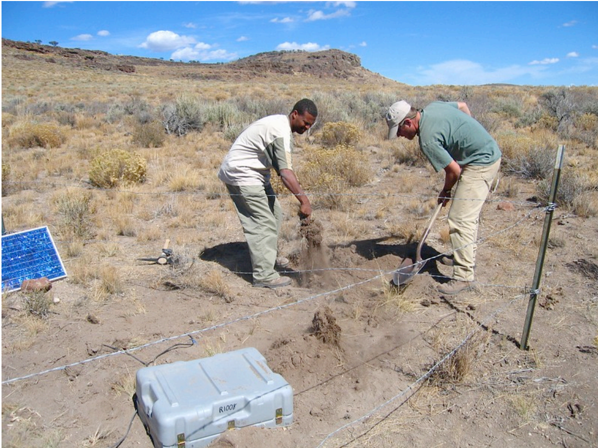
Example installation of passive seismometer (BLM Burns District, southeast Oregon), 2007. Note solar panel and GPS antenna remains on surface.
