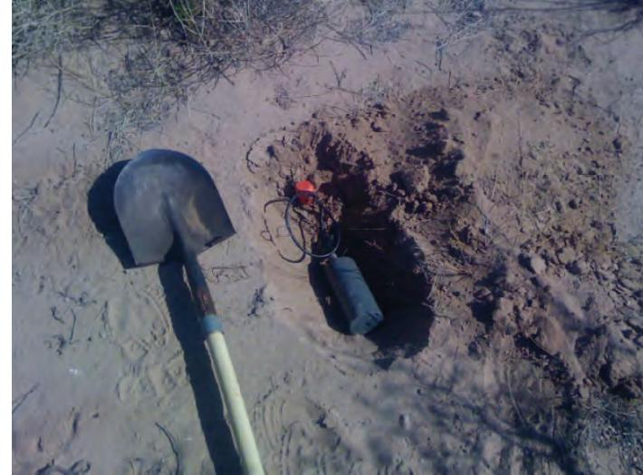
**Typical installation of a portable seismic monitoring system.** The recorder (grey steel cylinder) is connected to a geophone (orange plastic case on a short spike) that moves up and down as the earth moves up and down. Everything is buried in a small hole (see shovel for scale) to protect it from wind vibrations that can be much stronger than the earth vibrations we are monitoring.
