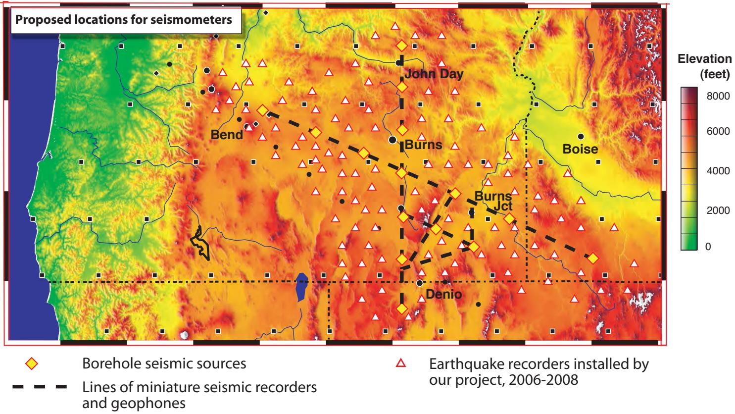
**Seismic Imaging** uses seismic waves to probe the earth beneath the stations. One method, called seismic “tomography”, is like a CAT scan of the human body. This is used to determine the hidden structures deep in the earth’s crust. Seismologists also use methods very similar to those used in oil and gas exploration that, together with tomography, will give a comprehensive picture of the earth’s structure beneath central and eastern Oregon, western Idaho, and northern Nevada.
