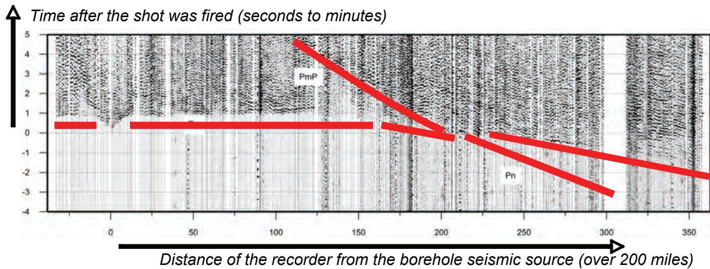
*We pick the arrival times of the seismic energy at each recorder ...
