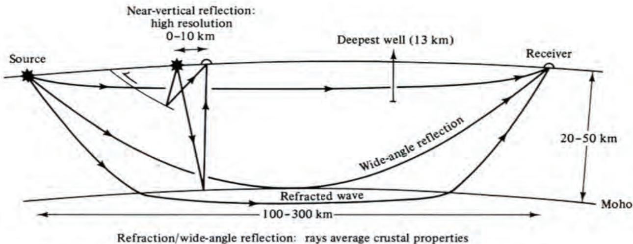
*The seismic waves spread out through the earth from the borehole detonation ...
