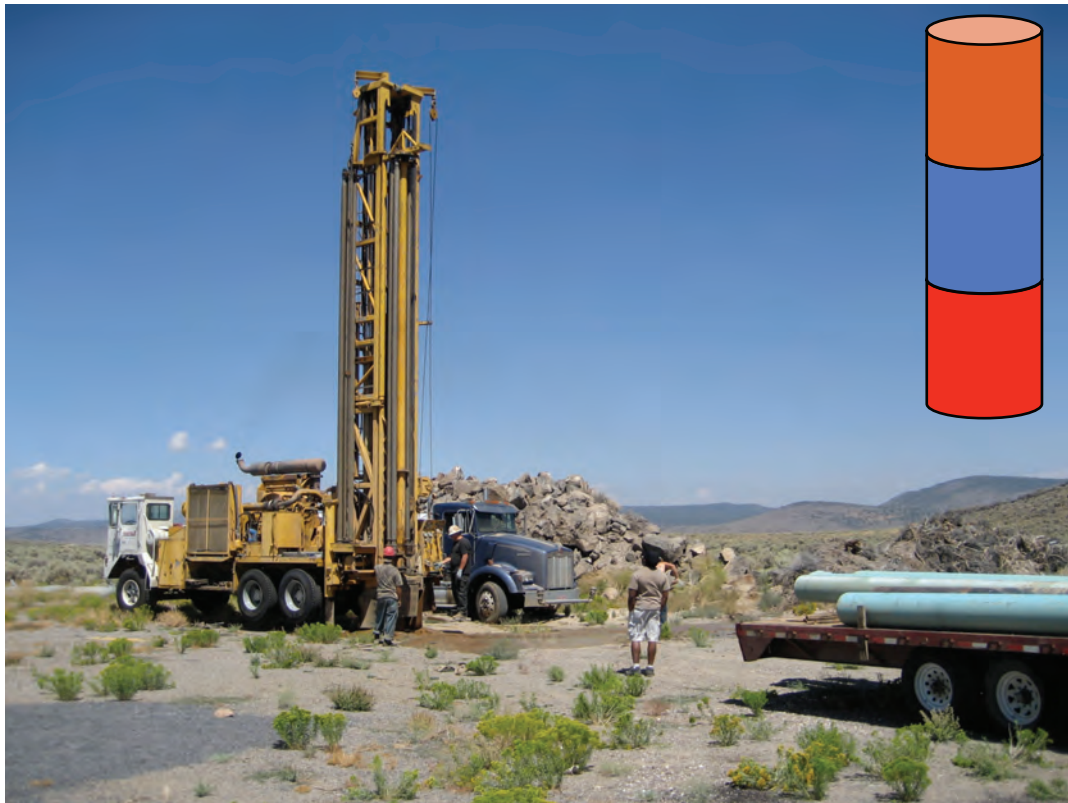
Figure 10. Field photo showing the drilling operations for the High Lava Plains Controlled- source seismic experiment. The shot holes were filled with 1-ton of emulsion gel (red), 60 ft of angular gravel (blue), and topped with cuttings and sediment (orange).
