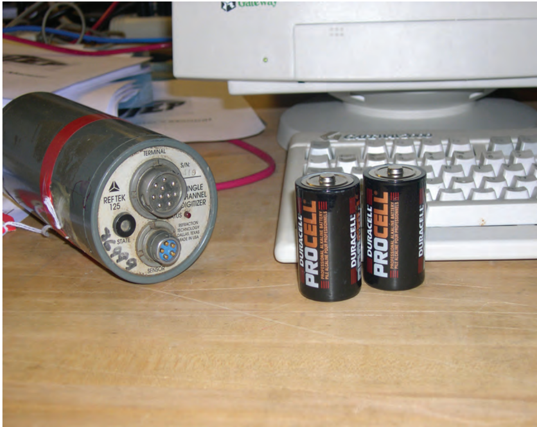
Figure 12. Photo of the Texan receivers used during the controlled-source experiment.
