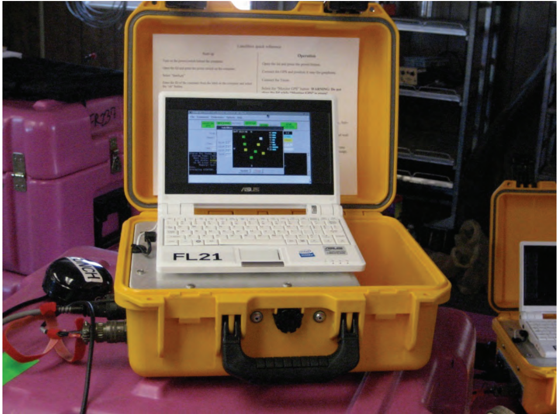
Figure 13. Photo of the “Lunchbox” used to record Texan locations.
