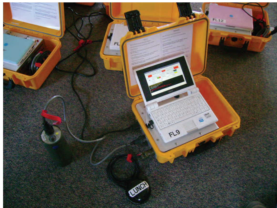
New "Lunch Box" used to take GPS readings in the field during deployment.
