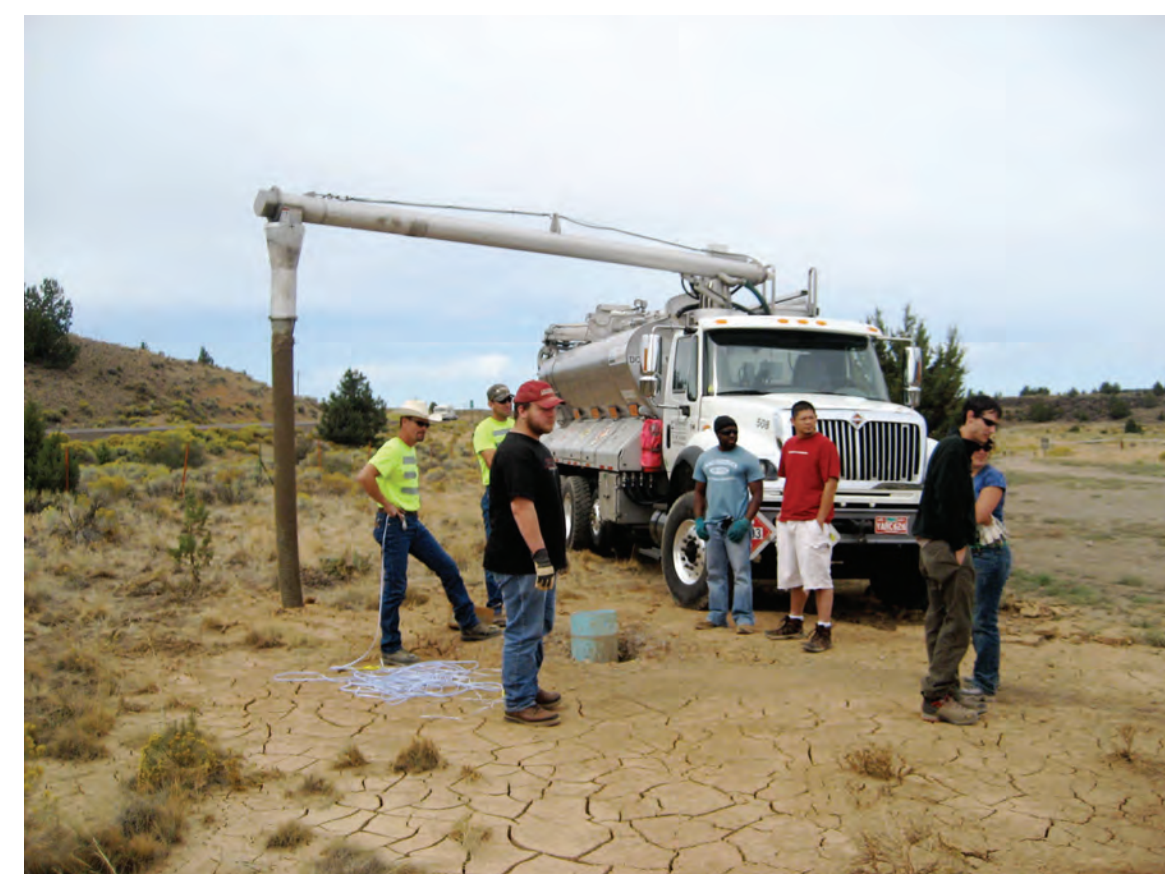
Loading of ammonium nitrate gel explosives.
