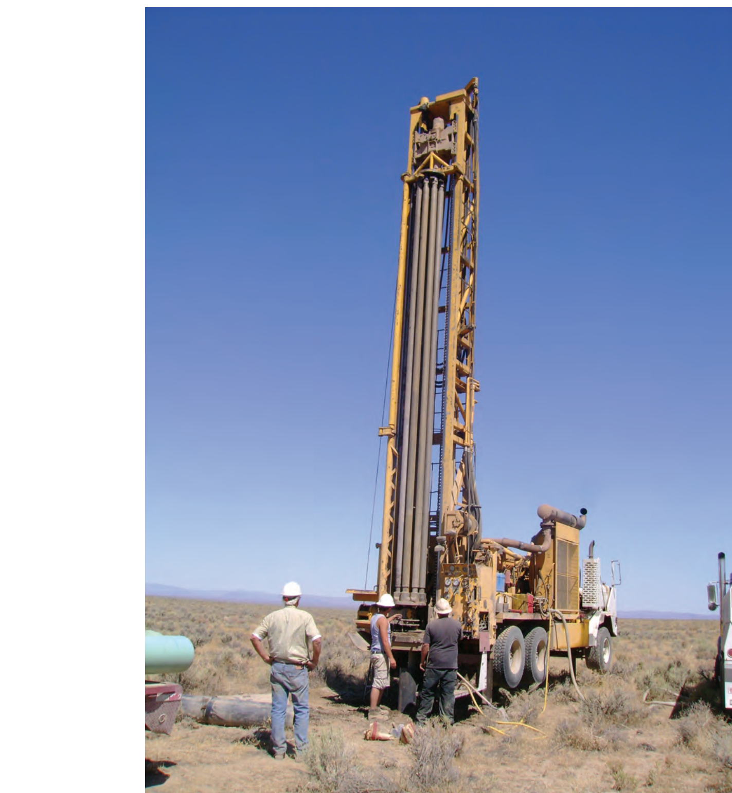
Drill rig used to drill 12 inch diameter hole to 80 feet deep.
