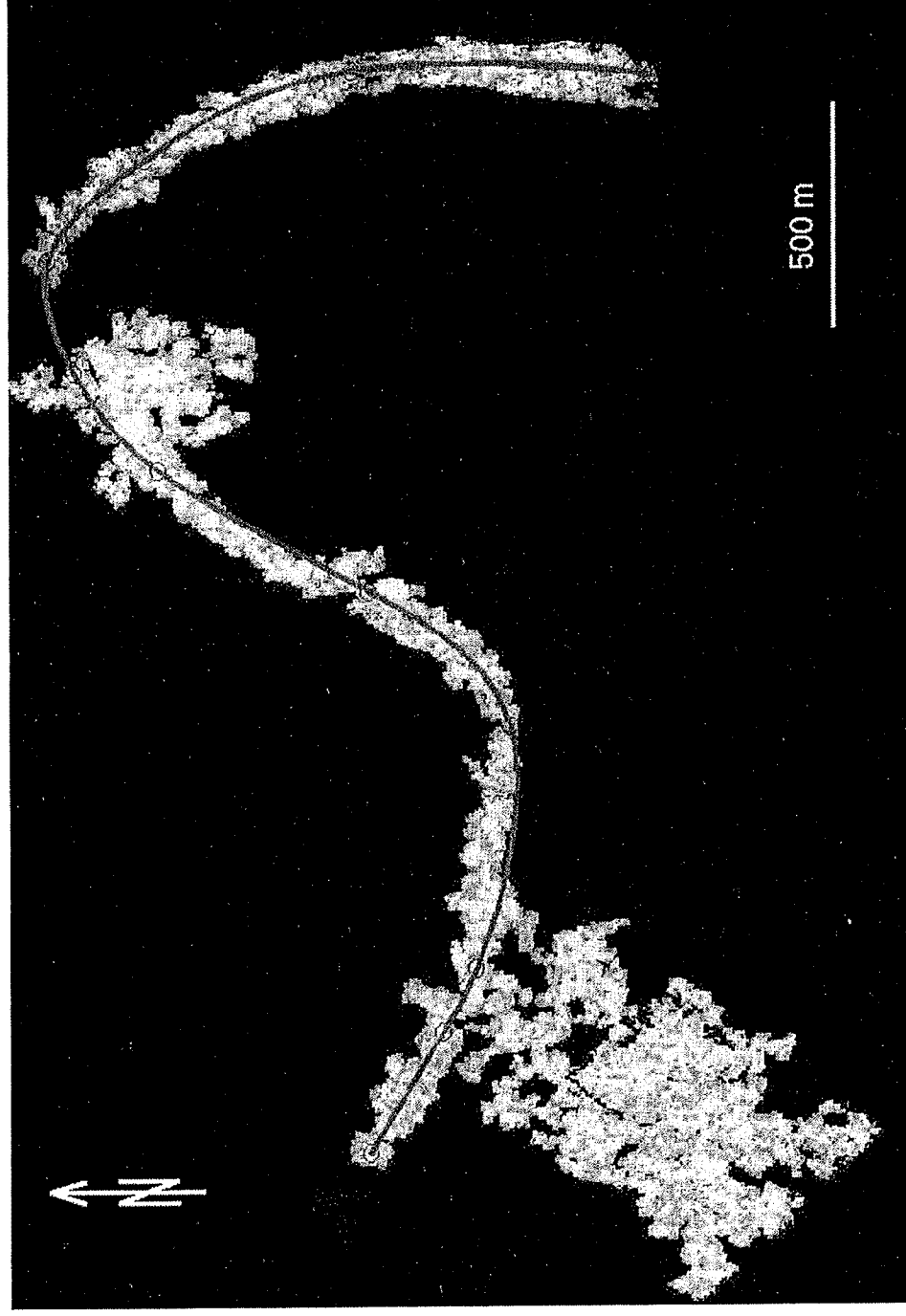
Fig. 4. Plan view of a channel with possible crevasse splays (left and top) extracted with the voxel-growing method.
