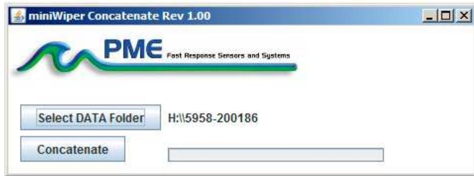
The miniWIPERConcatenate program reads and concatenates the files recorded by the miniWIPER. This program produces a CAT.txt file in the same folder as selected for the data. The CAT.txt file contains all the original measurements and contains two additional statements of time.
