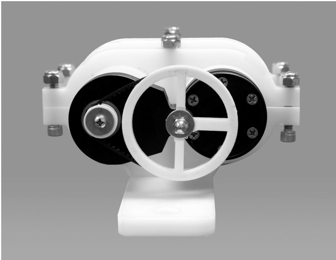
While maintaining the alignment (pictured above), slide miniWIPER and miniDOT Logger relative to each other until the brush engages the sensing foil as shown below. You may rotate the small pulley slowly by hand. This causes the internal motor to turn but will not damage miniWIPER. **DO NOT ROTATE THE LARGE PULLEY BUT INSTEAD ALLOW THE BELT TO MOVE THIS PULLY WHILE ROTATING THE SMALL PULLEY BY HAND. ROTATION OF THE LARGE PULLEY BY HAND CAN DAMAGE miniWIPER.**
