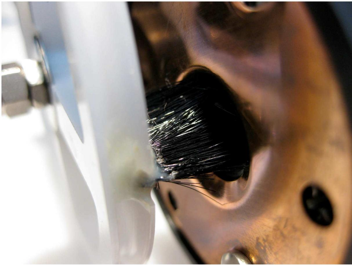
Tighten the 6 bolts while maintaining the miniWIPER and miniDOT positions. First tighten the 4 outer bolts until the gap in white plastic closes. Next tighten the inner two until the miniWIPER and miniDOT Logger are securely held. A small gap in white plastic on these inner bolts will remain when all is secure.
