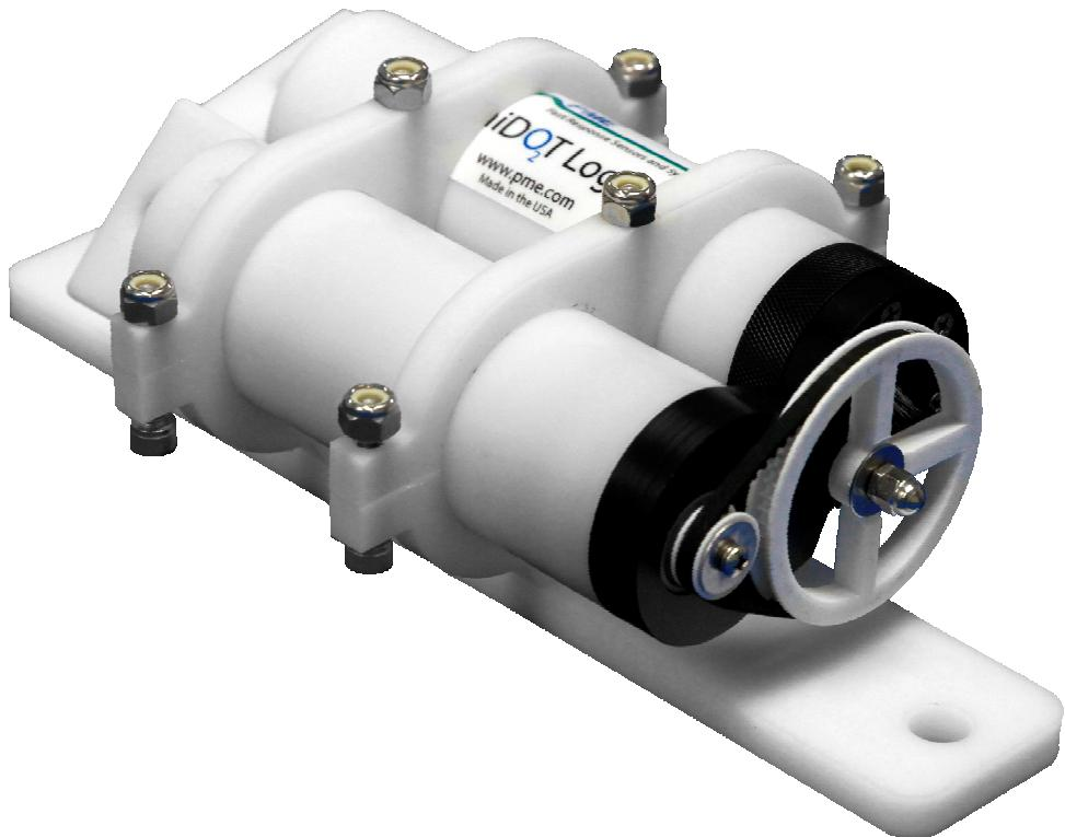
Rotate miniWIPER and miniDOT Logger until the miniDOT Logger sensing foil and the wiper pulley axes all align. There are two possible alignments, one with the sensing foil close to the wiper and one with the foil furthest away from the wiper. Select the alignment with the foil closest. The picture below shows the required alignment.
