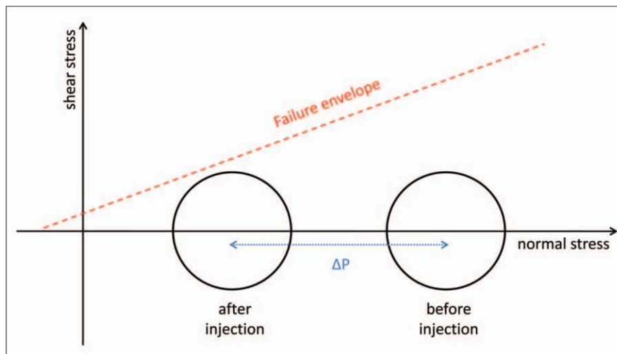
**Figure 3.** Mohr-Coulomb diagram illustrating how fluid injection lowers the normal stress and thereby brings rock closer to failure.
