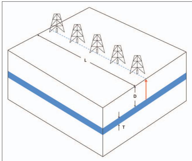
**Figure 4.** Schematic geometry of the hydrocarbon field in the poroelastic model for fluid extraction from a horizontal layer by Segall (1985). The producing horizon of thickness  $T$  is located at depth  $D$  and is assumed to be embedded in an impermeable half-space. Fluid is extracted homogeneously along the line of wells on the surface.
