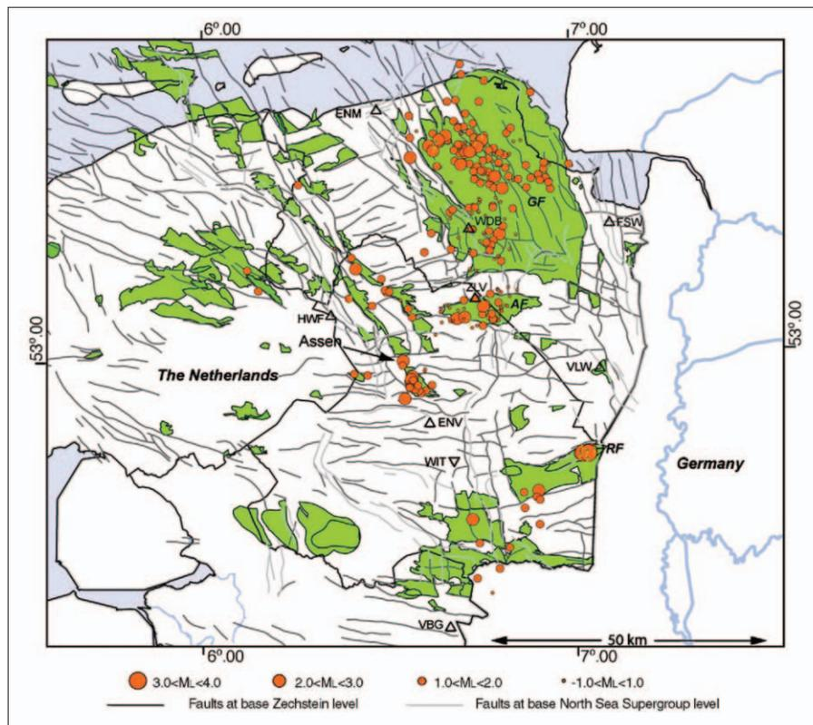
**Figure 2.** Illustration of the spatial correlation between hydrocarbon fields (green), major fault structures, and seismicity (solid orange circles) in the northeastern part of The Netherlands. The major gas fields are indicated: Roswinkel Field (RF); Groningen Field (GF), Eleveld Field (EF), Annerveen Field (AF). Seismic stations are shown as triangles. (Figure reproduced from Van Eck et al., 2006).
