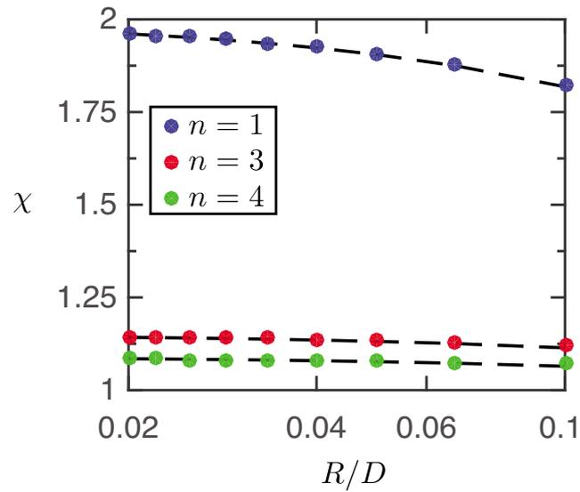
**Figure 3.** A plot of  $\chi$  against  $R/D$  for  $n = 1$ ,  $n = 3$ , and  $n = 4$ , alongside the fitting function  $\chi = \chi_{inf}(1+R/D)^{-1/n}$ . This plot allows us to infer values of  $\chi_{inf}$  that are then used to determine the maximum stress resolved on the undeforming bed. We find best fitting values of  $\chi_{inf}$  to be 2 for  $n = 1$ , 1.15 for  $n = 3$ , and 1.09 for  $n = 4$ .
