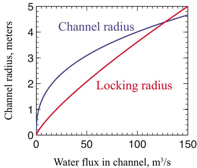
**Figure 6.** A plot of the channel radius  $R$  and locking radius  $R_{lock}$  against the water flux in the channel for the parameters in Tables 1 and 2 assuming a Glen’s law rheology. We see that  $R < R_{lock}$  – and thus a stable margin configuration exists – whenever the water flux exceeds a critical value of  $\sim 127$  m<sup>3</sup>/s. This water flux corresponds to a channel with a radius of 4 m.
