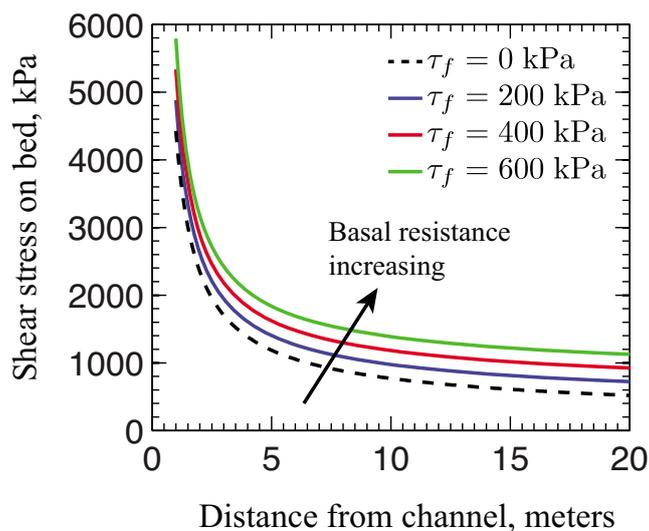
**Figure 5.** A plot showing how the stress on the undeforming bed varies with the basal resistance of the deforming bed  $\tau_f$  for the parameters in Table 1 and  $n = 1$ . Our results show that for these parameter choices the dependence of maximum stress on  $\tau_f$  is not significant. However, as discussed in Section 4.3, we expect the role of  $\tau_f$  to become more important as  $\tau_f$  becomes comparable to  $\tau_{sharp}(R)$ .
