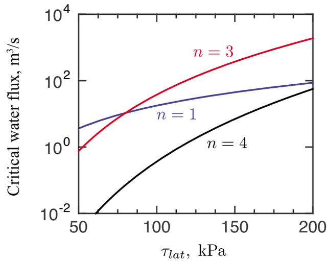
**Figure 8.** A plot of the critical water flux  $Q_{lock}$  against the average stress supported at the shear margin  $\tau_{lat}$  for  $n = 1$ ,  $n = 3$ , and  $n = 4$ . This plot was produced using the parameters in Tables 1 and 2. We see that  $Q_{lock}$  increases rapidly with  $\tau_{lat}$ . Note that the  $n = 4$  curve predicts much lower critical water fluxes than  $n = 1$  and  $n = 3$ .
