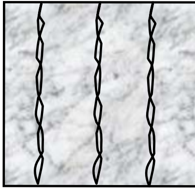
Figure 2.9: Graphical representation of the fractures modeled with a planar distribution of circular welded regions.
