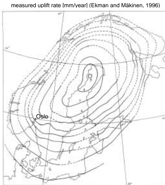
Figure 4.20: Map of apparent uplift rates in Fennoscandia (Ekman, 1996). The map is based on the compilation of sea level recordings, lake level recordings, and high-precision leveling between 1892 and 1991. The shown values are apparent uplift rates (relative to sea level).
