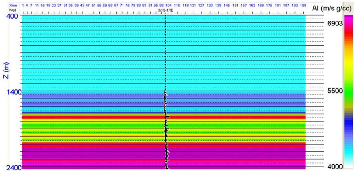
Figure 7.7: Initial model of acoustic impedance (m/s g/cc) section in depth, generated only from well information. Well is at center of the section.
