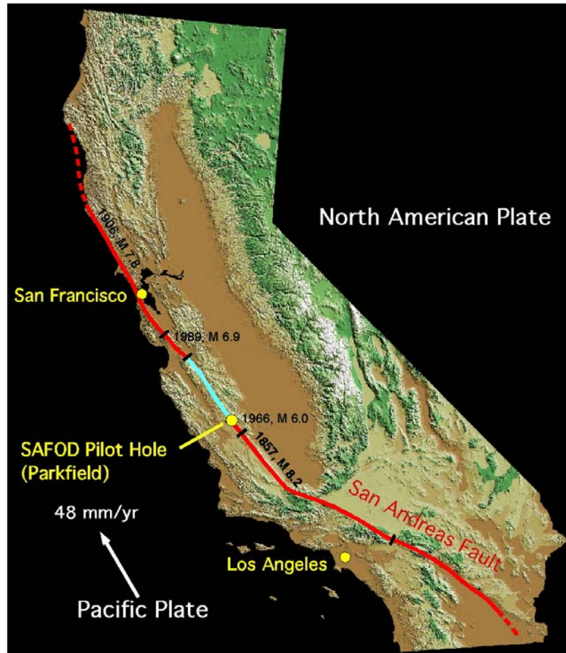
Fig 2.1: The SAFOD borehole is located at Parkfield on a segment of the SAF that shows aseismic creep and repeating micro earthquakes.
