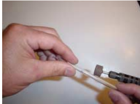
Figure P2: Scoring sample tubes using file (left photo) or the Dremel Tool. With either technique it is necessary to make a score completely around the glass sample tube. Also, care should be taken not to break the glass sample tube or cutting your hand. With the file technique (left photo) apply enough pressure with your thumb to allow the file to cut into the glass while also allowing you to rotate the sample tube with the opposite hand. When using the Dremel Tool (right photo) set the Variac controller on 20 to 25 (out of 100), press the sample tube against grinding wheel and rotate making a score completely around the sample tube.
