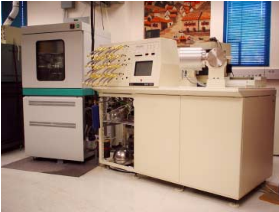
Stanford University Stable Isotope Laboratory Finnigan MAT252 mass spectrometer with 24 port manifold, and Kiel II carbonate device.
