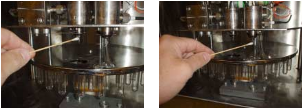
Figure P4: Clean the acid drip counters and capillaries on both Port 1 (left photo) and Port 2 (right photo) using 2-propanol and a cotton swab. Extra care should be taken not to alter the alignment between the counter and capillary.
