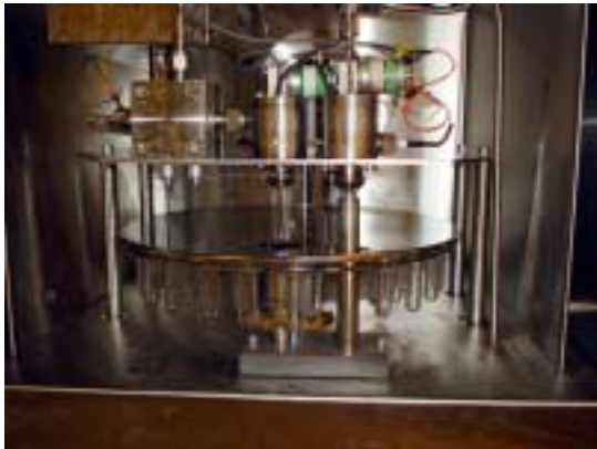
Figure P6: Reloading the sample vials after cleaning and greasing Ports 1 and 2 (top left to bottom right).
