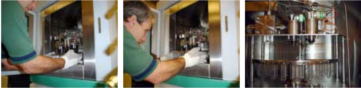
Figure P3: Removing and installing the sample carousel on the Finnigan Kiel III. To remove, carefully lift the carousel to free the shaft from the pivot base (left photo). Slide carousel out without touching the capillaries, counters, or pistons with the carousel or vials. To install, taking the same precautions as above, carefully slide the carousel in and gently place the carousel shaft onto the pivot base (middle photo). You will need to align the pin on the carousel shaft with the slot on the pivot base as well as the slot on the carousel top shroud with the vertical rod at the back of the unit (right photo).
