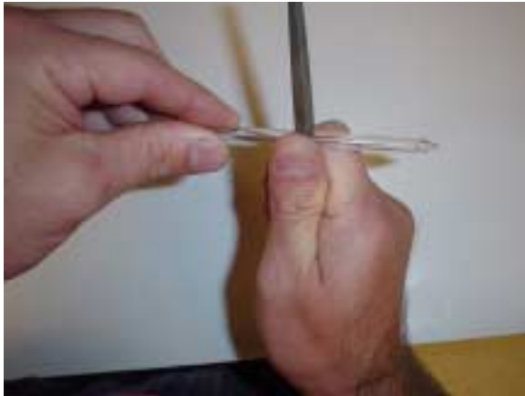
Figure P2: Scoring sample tubes using file (left photo) or the Dremel Tool. With either technique it is necessary to make a score completely around the glass sample tube. Also, care should be taken not to break the glass sample tube or cutting your hand. With the file technique (left photo) apply enough pressure with your thumb to allow the file to cut into the glass while also allowing you to rotate the sample tube with the opposite hand. When using the Dremel Tool (right photo) set the Variac controller on 20 to 25 (out of 100), press the sample tube against grinding wheel and rotate making a score completely around the sample tube.
