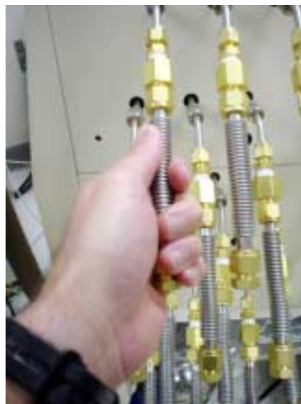
Figure P4: After you press measure (F5) you need to crack all sample tubes. It is best to do this in an orderly manner so you do not miss any samples. Crack sample tubes by bending the bellows tube until you hear the glass sample tube break (right photo).
