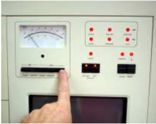
Figure P1: Perform a fore vacuum check by pressing the black FV Inlet button on the far right and monitor by reading the lower green bar (left photo). When finished press the black HV source button on the far right and monitor by reading the upper red bar (right photo).
