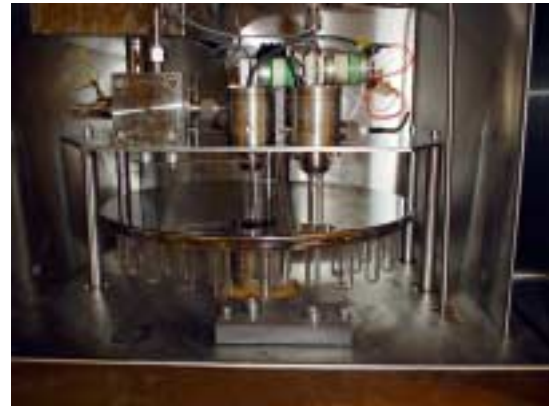
Figure P6: Reloading the sample vials after cleaning and greasing Ports 1 and 2 (top left to bottom right).
