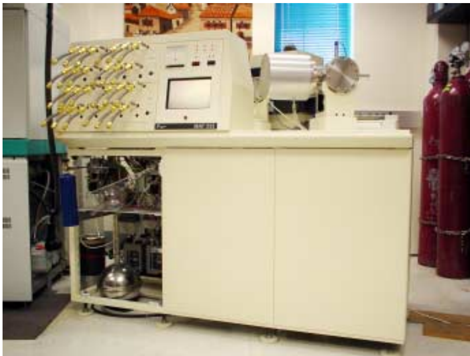
Stanford University Stable Isotope Laboratory Finnigan MAT252 mass spectrometer with dual inlet and 24 port manifold.
