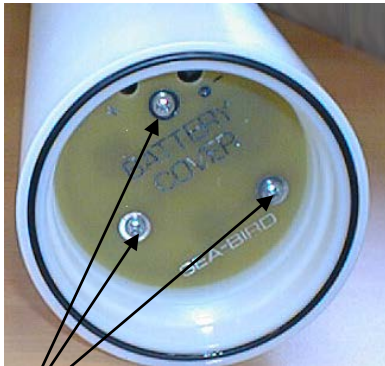
Remove Phillips-head screws and washers
