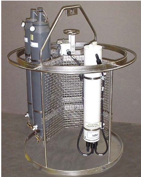
With one 3-position lanyard release module and 3 bottles
