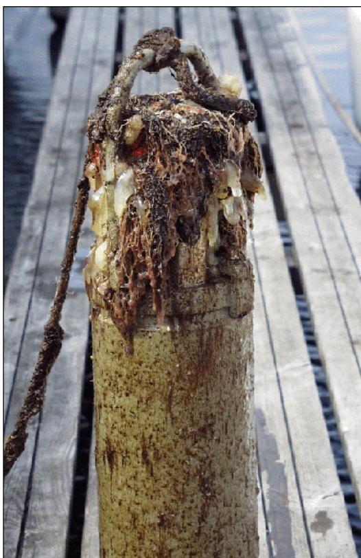
Figure 20 Example of fouling on an RCM 9 Mk II with an Oxygen Optode 3830 mounted to it: The Optode was still giving correct readings.
