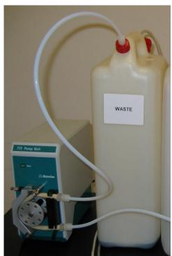
M8 tubing-Attach to Aspiration Tip
