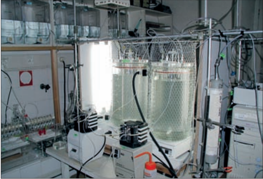
Figure 5.3 Chemostat used by Sciandra et al. (2003) to investigate the response of Emiliana huxleyi to elevated p(\text{CO}_2) (photo credit: J.-P. Gattuso).
