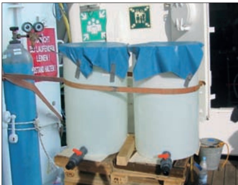
Figure 2.1 Aeration system for seawater carbon dioxide ( \text{CO}_2 ) enrichment consisting of a bottle of pure \text{CO}_2 gas and two 250 l seawater containers (photo credit: K. Schulz).
