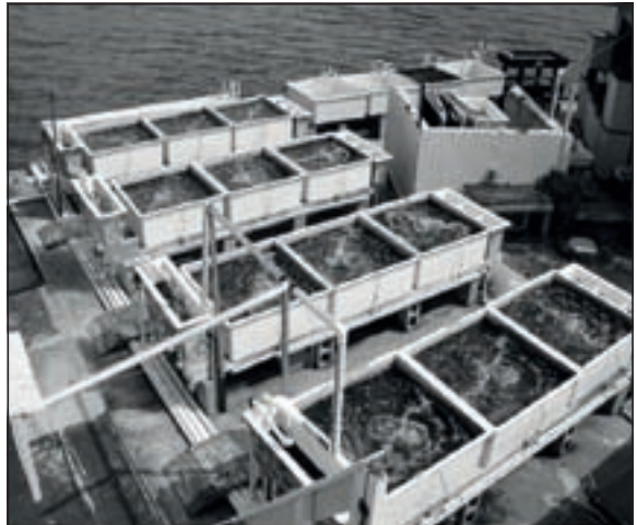
Figure 13.3 Outdoor continuous-flow mesocosms for studying the long term impacts of ocean acidification on coral reef organisms at the Hawaii Institute of Marine Biology (HIMB) (used with permission from Andersson et al. , 2009).
