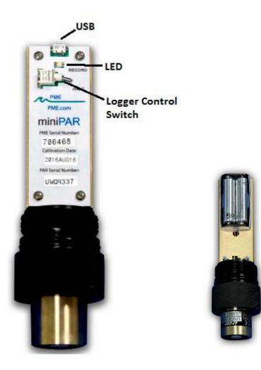
The **LED Light** is a LED that can display either red or green light. This is used to indicate the different features described in Chapter 1 in this manual.
