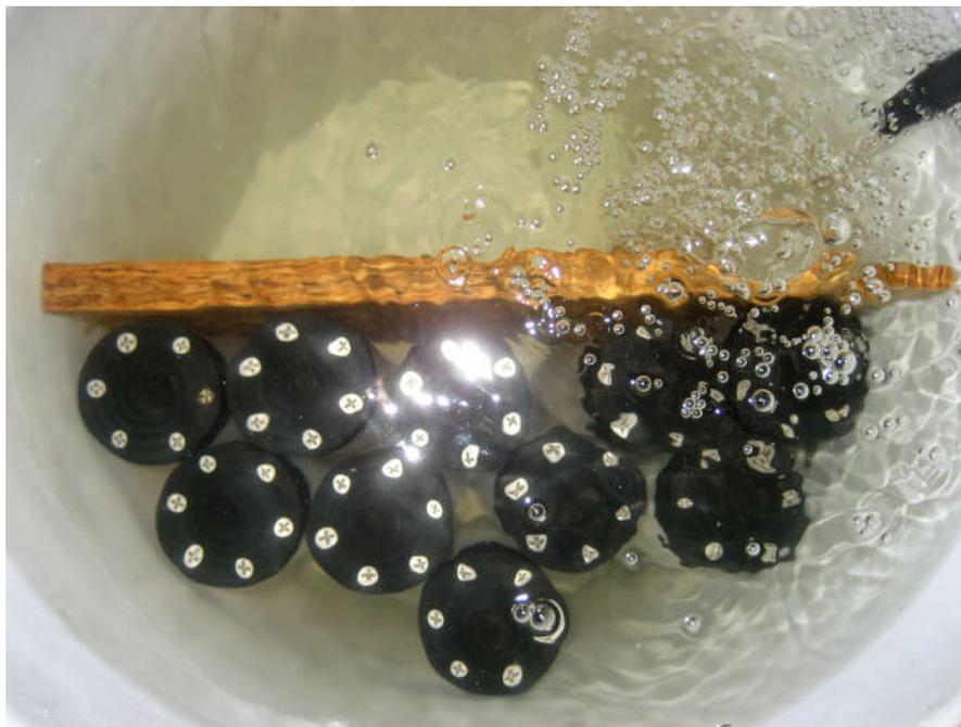
Record measurements for several hours or a day, but in any event long enough for the miniDOT Logger's temperature to come to equilibrium with the water. During the experiment,
