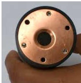
4. Install the three pan head screws included in the kit. Gently tighten.
