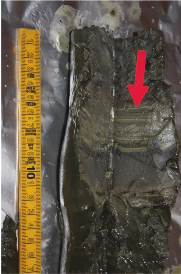
Fig. 7.8 Detailed view of sediment core from Lake Caviahue showing laminations unchanged (red arrow), which indicates the lack of bioturbation
