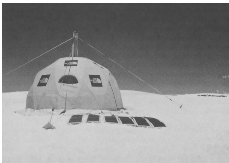
Figure 3. The new portable 3-inch electromechanical drill installed in a sheltering tent and powered by flexible solar panels in operation on the cerro Tapado ice cap.
