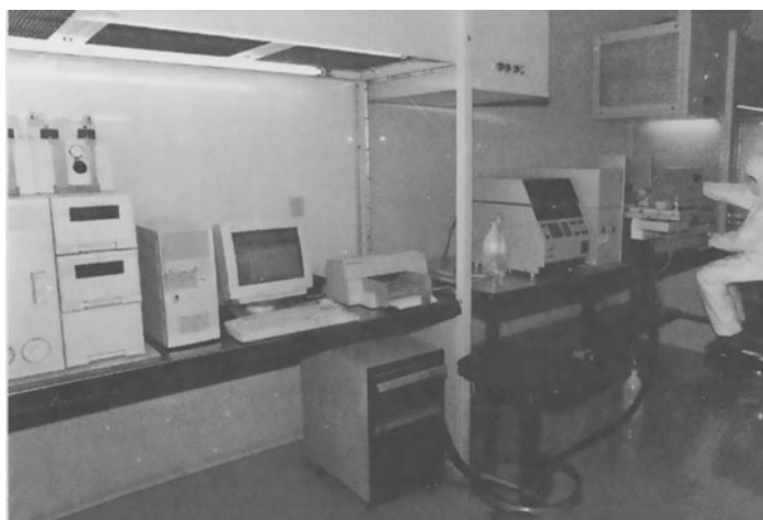
Figure 2. View of the ion chromatograph and the atomic absorption spectrophotometer, to measure ionic concentration of the samples, in the clean chamber of the LEGAN.
