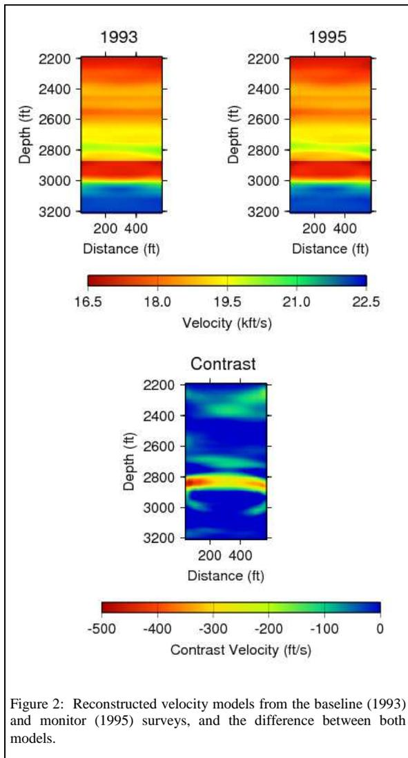
Figure 2: Reconstructed velocity models from the baseline (1993) and monitor (1995) surveys, and the difference between both models.
