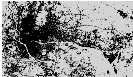
Figure 3.12: Reference binary image of impervious (black) versus non-impervious (light grey) surfaces for the city of Guangzhou, China. Image extent: 735 \times 420 fine pixels.
