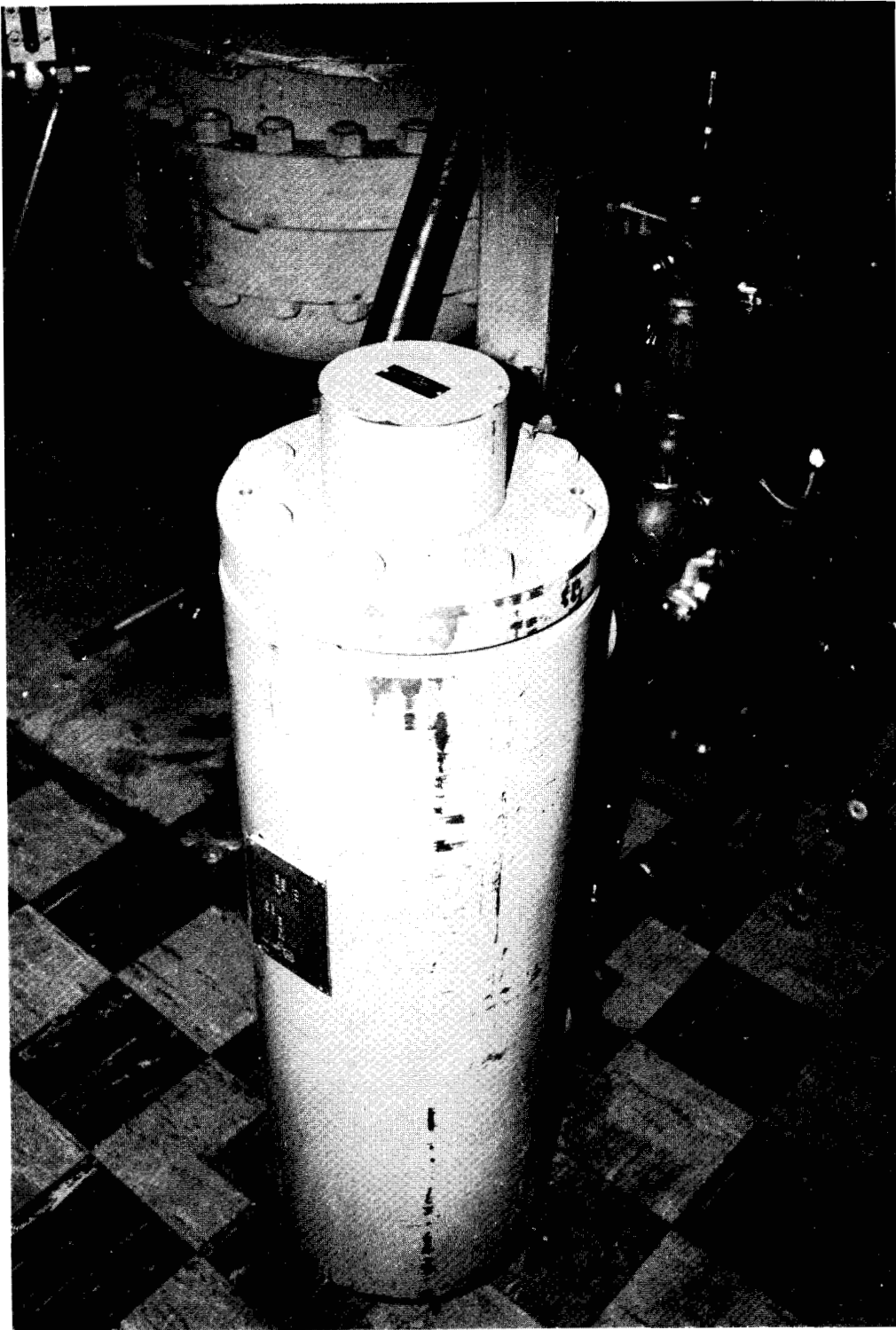
Figure 2.6 Side view of chimney model system with the electric circulation heater in the foreground prior to installation of insulation
