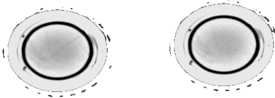
Figure 1.1: CT dry scan (left) and CT wet scan (right). From average values within the core, CT_{dry}=1486 CT_{wet}=1511 .
