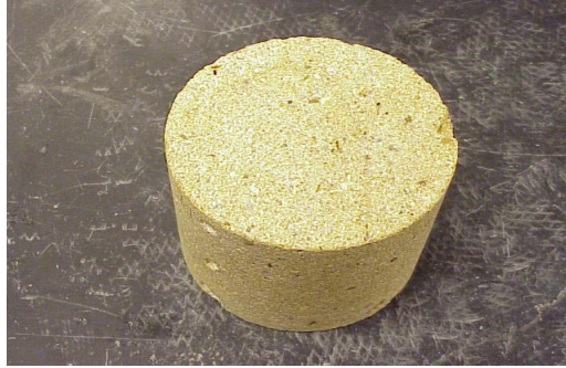
Figure 4.5: the heterogeneous shaly sandstone core.
