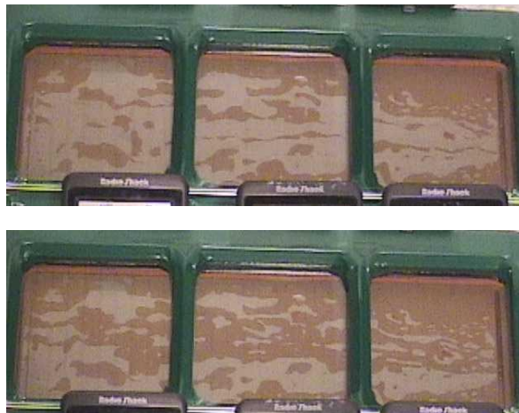
Figure 1.9 Examples of gas flow path increase in width as gas flow rate increases and water breaking up this flow path.
