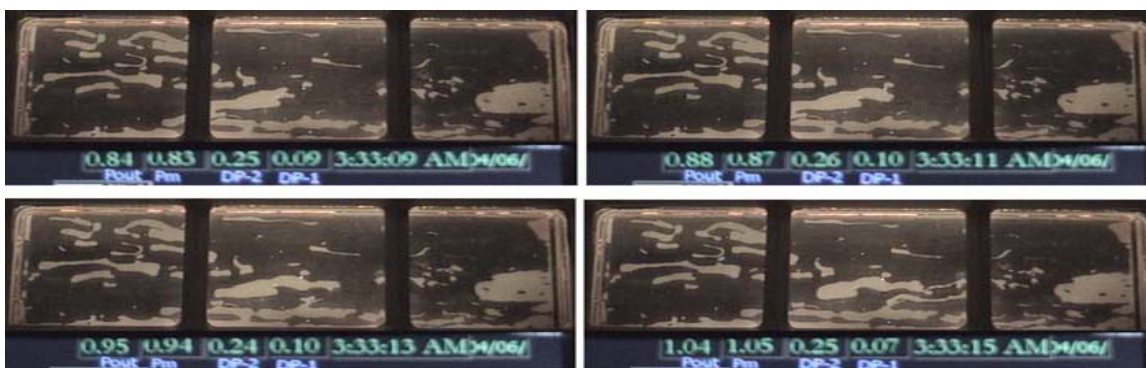
Figure 1.26: The continuous nitrogen-water flow behavior in smooth-walled fracture at room temperature under low water saturation ( \sim 15\% ) (nitrogen phase is dark, water phase is light, Q_w=0.5\text{ml/min} , Q_g=200\text{ml/min} ).
