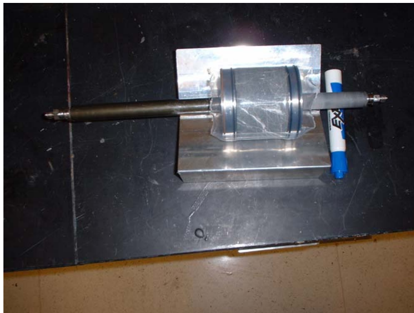
Figure 5.2: Photo of the geothermal core with shrink tubing and end plates
