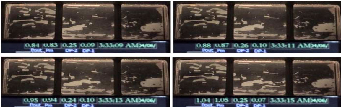
Figure 1.26: The continuous nitrogen-water flow behavior in smooth-walled fracture at room temperature under low water saturation (~15%) (nitrogen phase is dark, water phase is light, Q_w=0.5\text{ml/min} , Q_g=200\text{ml/min} ).
