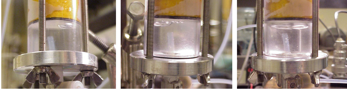
(a) Bubble forms (b) Bubbles form and expand (c) Gas cap
