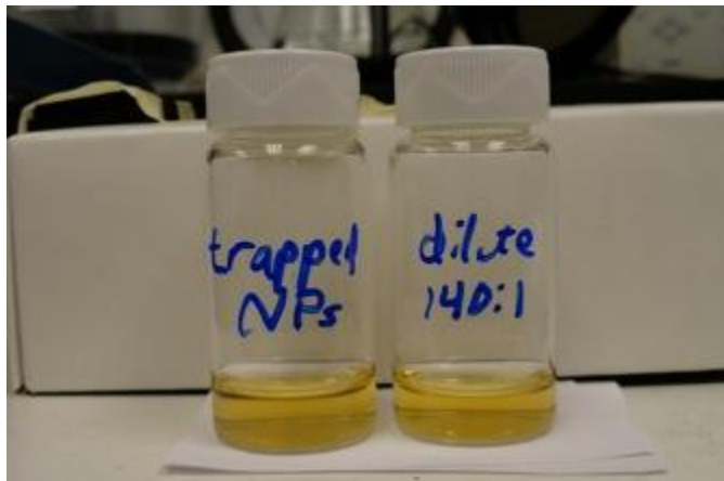
Figure 2.16: Visual comparison of trapped nanofluid sample and 142.5 to 1 dilution of original nanofluid.
