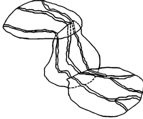
Figure 1.36: A conceptual channeling model of three intersecting fractures taken from Tsang and Neretnieks (1998).
