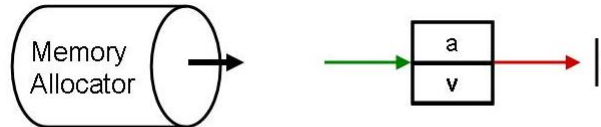
(a) The only overloaded SPLC operator that requires dynamic memory allocation is a constant times a sparse vector, c.v
