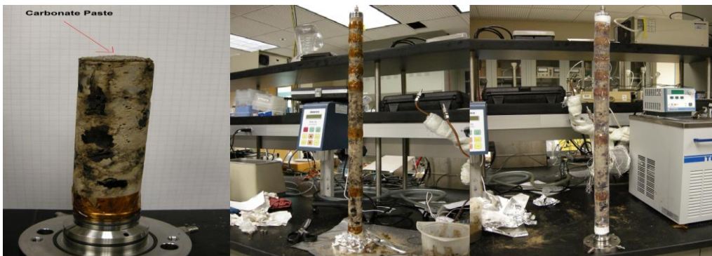
Figure 5-7: Carbonate paste. Figure 5-8: Aligned cores. Figure 5-9: Coated cores.
