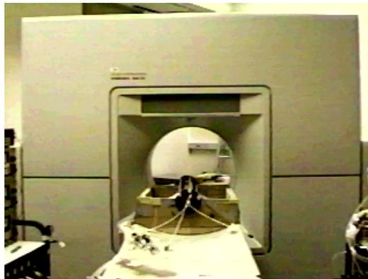
*Figure 1.1: A picture of the X-ray CT scanner and the core holder used in flow experiments*
