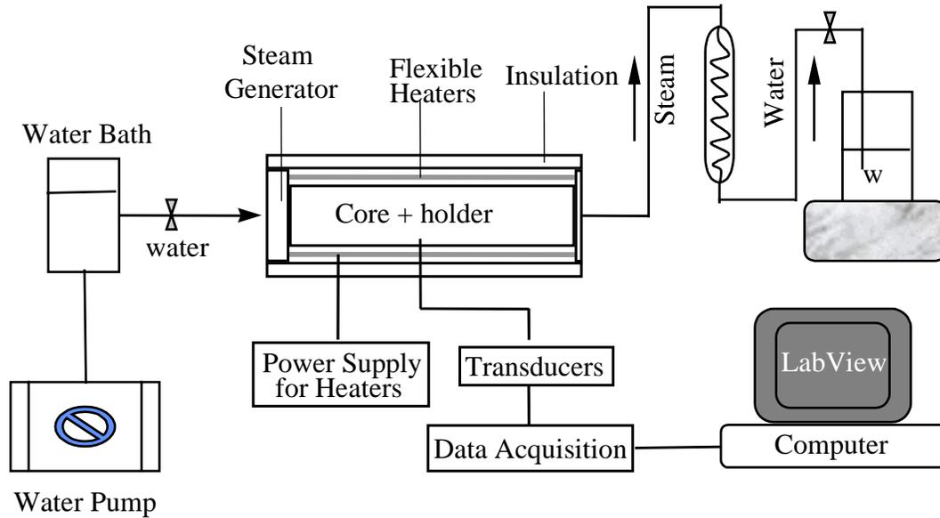
Figure 5.4: Schematic of apparatus for measuring steam slip factor using flexible heaters.
