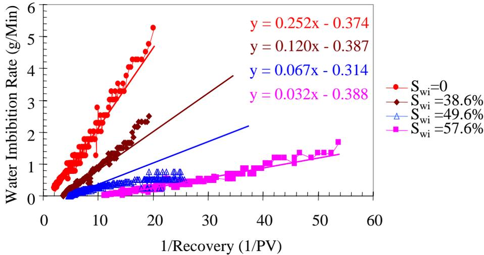
Figure 4.10: Water imbibition behavior at different values of initial water saturation in a sandstone sample.
