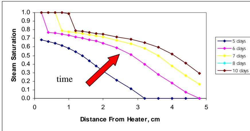
Figure 3.5: Steam saturation profile: endpoint water saturation = 0.2.
