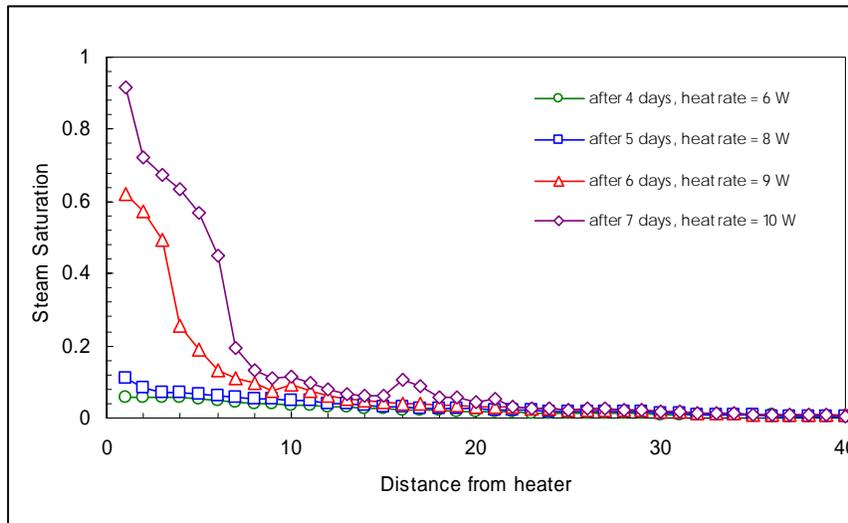
Figure 3.9: Steam saturation profile: bottom-heating vertical boiling experiment, Satik, Summer 1997.
