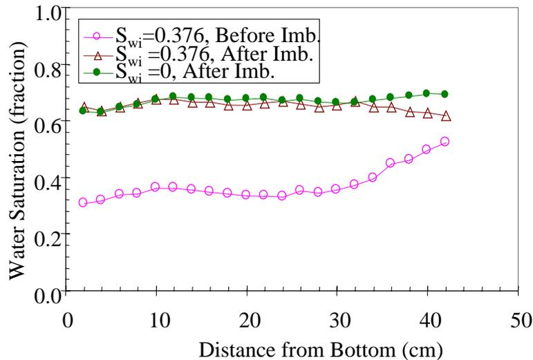
Figure 4.12: Distributions of water saturation in a sandstone core.
