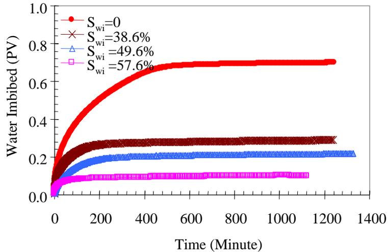
Figure 4.9: Water gain vs. time in sandstone at different initial water saturation.
