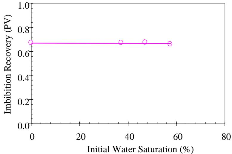
Figure 4.14: Imbibition recovery vs. initial water saturation in a sandstone sample.
