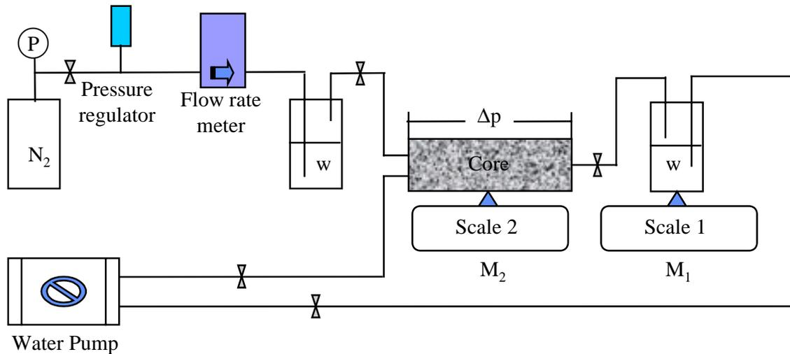
Figure 4.2: Schematic of gas-water relative permeability steady-state test.
