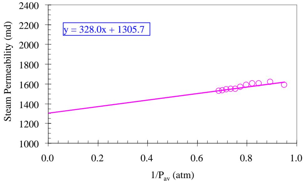
Figure 5.10: The slip factor of steam in the core with permeability of 1460 md at a temperature of 120°C.
