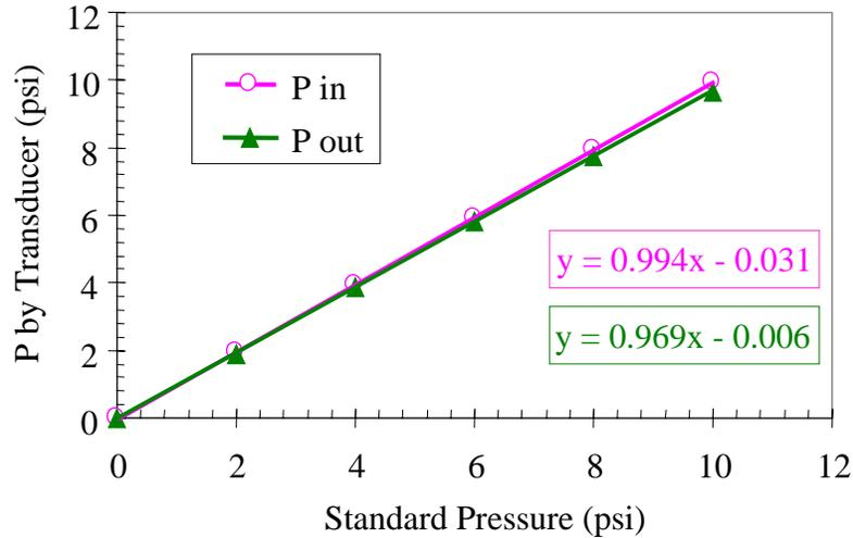
Figure 5.5: Calibration of pressure transducers at inlet and outlet.
