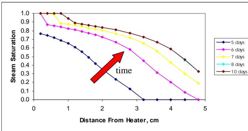
Figure 3.4: Steam saturation profile: endpoint water saturation = 0.1.
