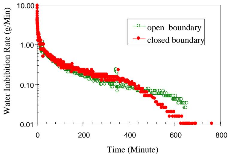
Figure 4.4: Water imbibition rate vs. time in sandstone.
