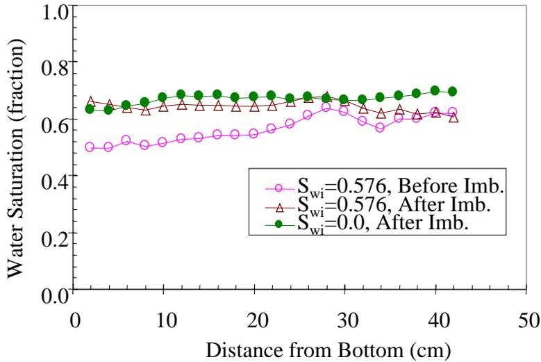
Figure 4.8: Distribution of water saturation in a sandstone sample by using a steady state technique.
