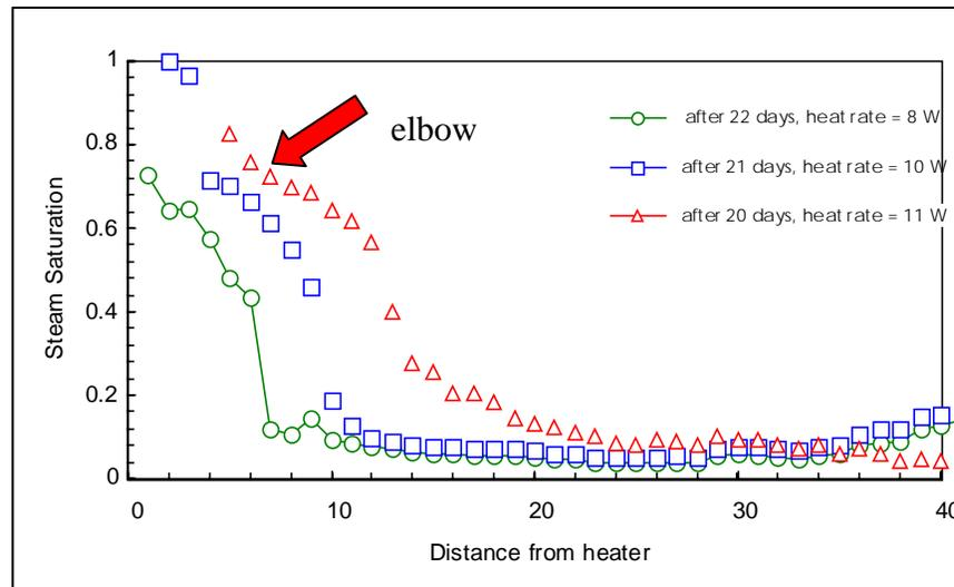
Figure 3.2: Steam saturation profile vertical boiling experiment, Satik, Spring 1997.
