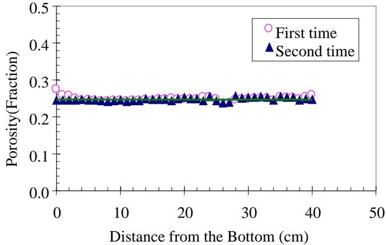
Figure 1.1: Porosity distribution along the core.
