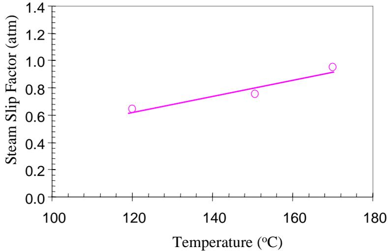
Figure 5.7: Relationship between steam slip factor and temperature.
