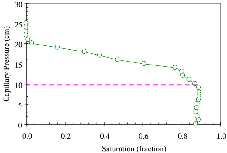
Figure 4.16: Air-water imbibition capillary pressure of a glass-bead pack measured using the X-ray CT technique.
