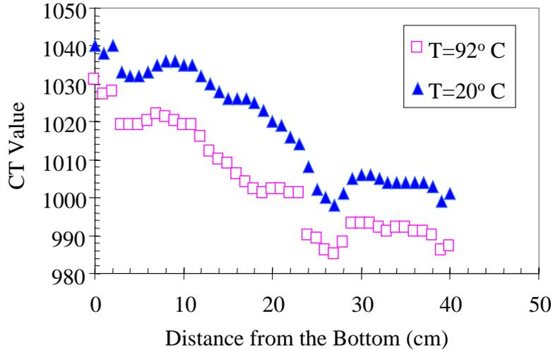
Figure 1.2: Effect of temperature on the values of  $CT_{dry}$ .
