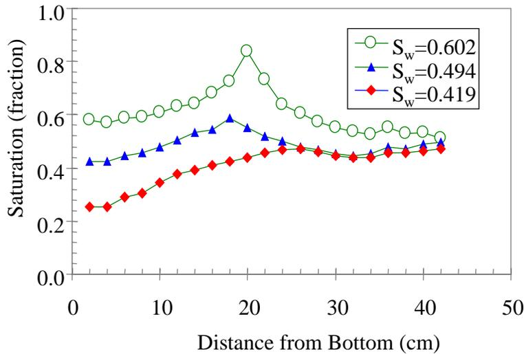
Figure 4.7: Distribution of water saturation in a sandstone sample by using single air injection.
