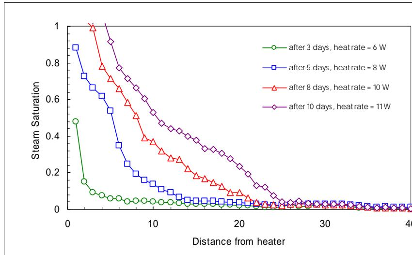
Figure 3.7: Steam saturation profile horizontal boiling experiment, Satik, Summer 1997.
