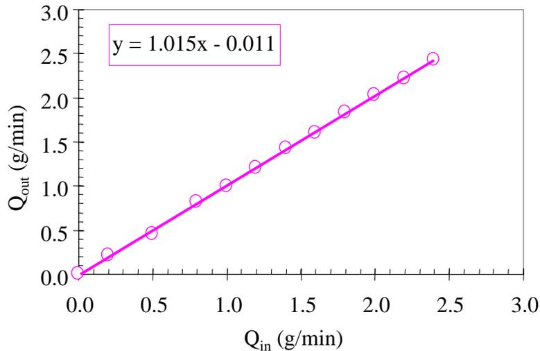
Figure 5.8: The comparison of the steam flow rates at the inlet with those at the outlet of the core.
