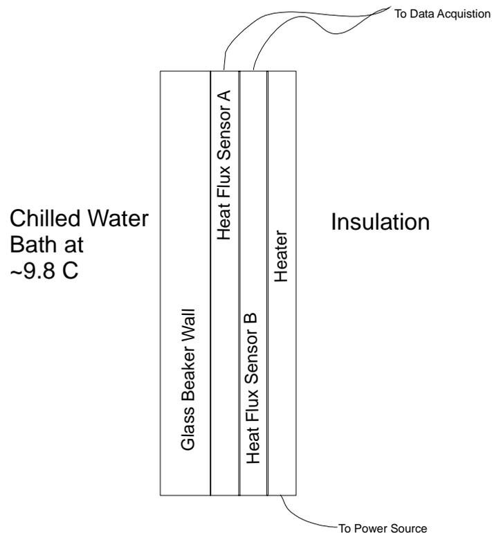
*Figure 2.1: Heat flux sensor  $k$  calculation experiment.*
