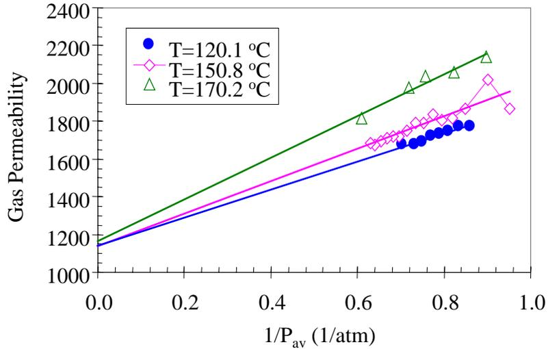
Figure 5.6: Effect of temperature on steam permeabilities and slip factor.
