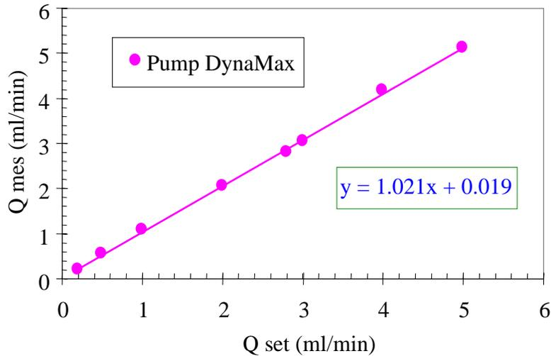
Figure 5.2: Calibration of flow rate for DynaMax pump.
