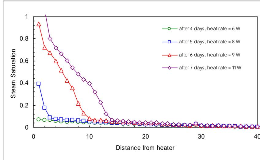
Figure 3.8: Steam saturation profile: top-heating vertical boiling experiment, Satik, Summer 1997.
