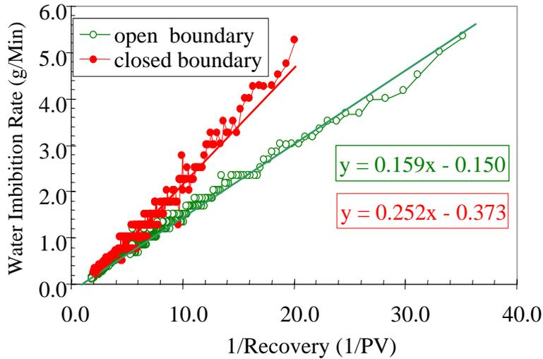
Figure 4.5: Water imbibition rate vs. reciprocal of production in sandstone.
