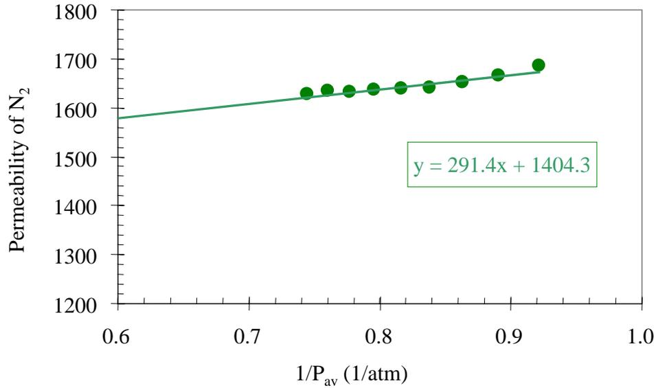
Figure 5.9: The slip factor of nitrogen in the core with permeability of 1460 md at room temperature.
