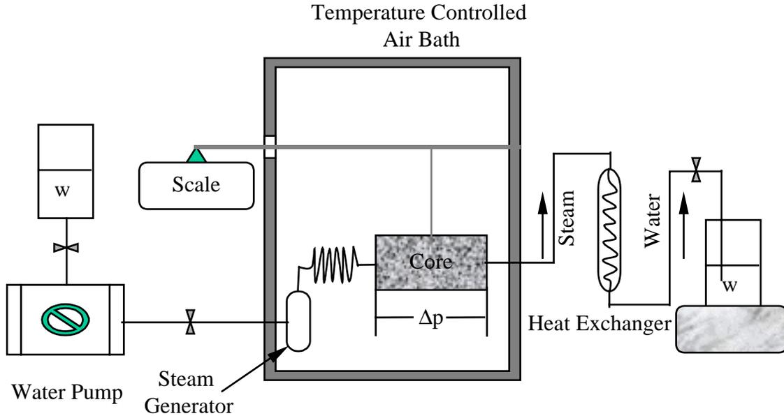
Figure 5.1: Schematic of apparatus for measuring steam slip factor.
