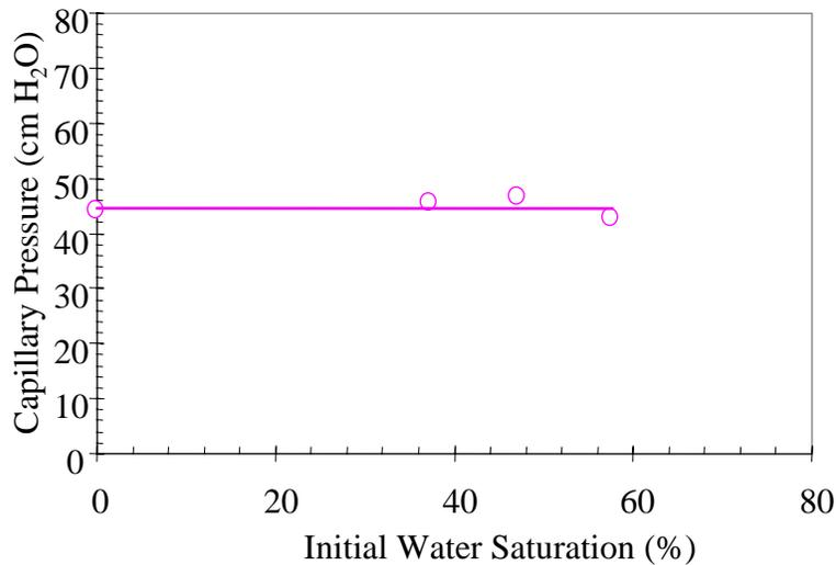
Figure 4.13: Capillary pressure vs. initial water saturation in a sandstone sample.
