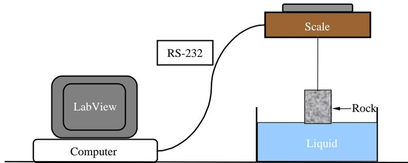
*Figure 4.1: Schematic of apparatus for imbibition test.*
