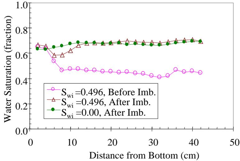
Figure 4.11: Distributions of water saturation in a sandstone core.
