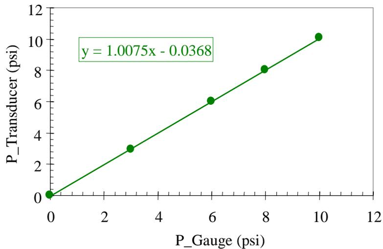
Figure 5.3: Calibration of differential pressure transducer.
