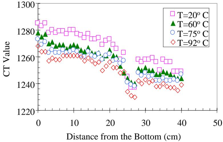
Figure 1.3: Effect of temperature on the values of  $CT_{wet}$ .
