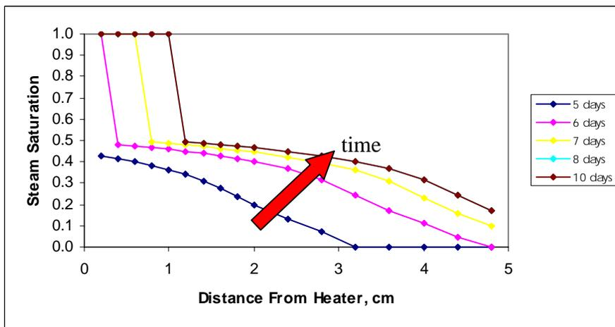
Figure 3.6: Steam saturation profile: endpoint water saturation = 0.5.
