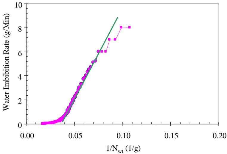
Fig. 4.15: Water imbibition rate vs. reciprocal of production in a glass-bead pack.
