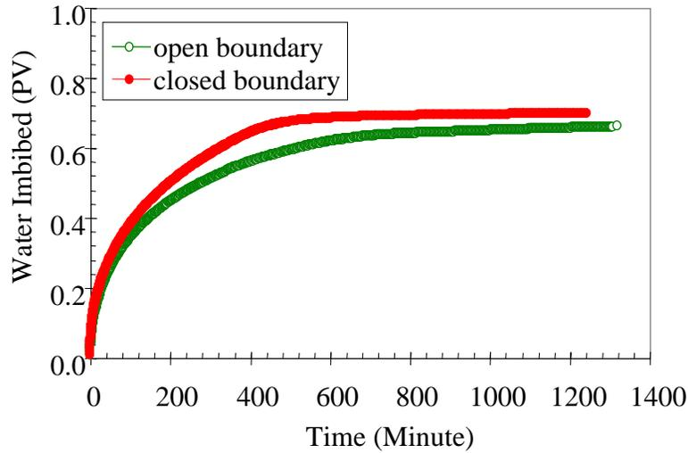
Figure 4.3: Water imbibition vs. time in the core at different boundary conditions.
