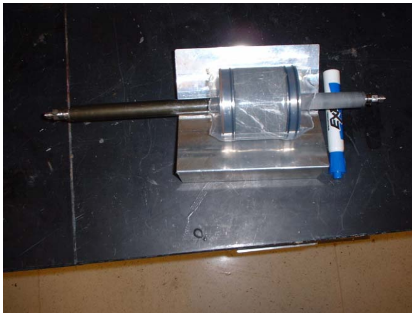
Figure 3-2: Photo of the geothermal core with shrink tubing and end plates
