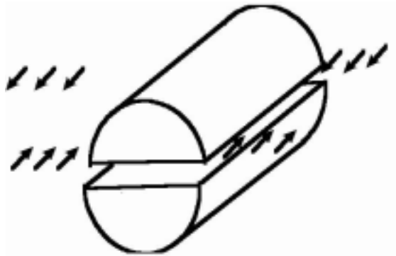
Two shim stock slide in along the arrows Figure 3.1: Experimental setup
