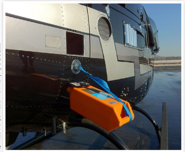
FIGURE 1 28 V Li-ion aircraft battery.
