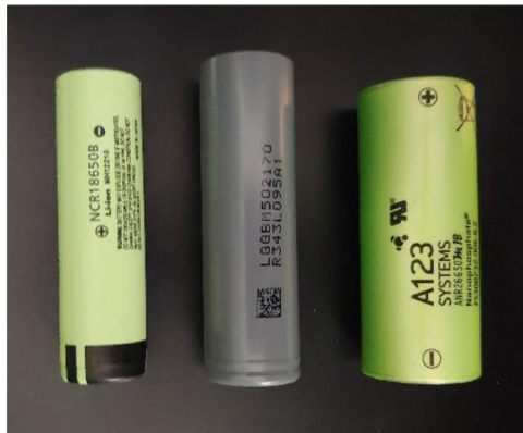
Fig. 1. Cell sample of NCA, NMC and LFP battery (from left to right) used in this work.
