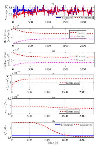
Fig. 5. Performance evaluation of the interconnected adaptive observer for the US06 drive cycle of Cell # B. (a) Voltage estimation compared with experimental data. (b)–(e) Estimation of bulk, surface concentration, diffusion coefficient, and conductivity in the SEI layer, respectively. (f) Capacity estimation validated against the measured capacity. Error in capacity estimate is less than 2%.
