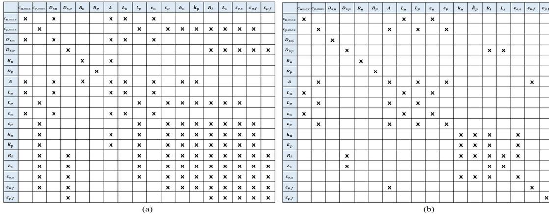
Fig. 11. Correlation analysis for ESPM parameters for (a) single-objective function and (b) multiobjective function. The times symbol (x) represents the values of  $\hat{C}_{i,j} > 0.8$  and, hence, indicates that parameters are correlated.
