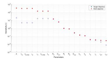
Fig. 10. Ranked sensitivity comparison for EPSM parameters with single-objective and multiobjective optimization functions.
