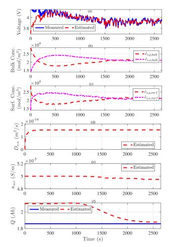
Fig. 6. Performance evaluation of the interconnected adaptive observer for the UDDS drive cycle of Cell # B. (a) Voltage estimation compared with experimental data. (b)–(e) Estimation of bulk, surface concentration, diffusion coefficient, and conductivity in the SEI layer, respectively. (f) Capacity estimation validated against the measured capacity. Error in capacity estimate is less than 2%.
