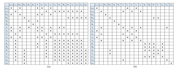
Fig. 11. Correlation analysis for ESPM parameters for (a) single-objective function and (b) multiobjective function. The times symbol ( $\times$ ) represents the values of  $\bar{C}_{i,i} > 0.8$  and, hence, indicates that parameters are correlated.
