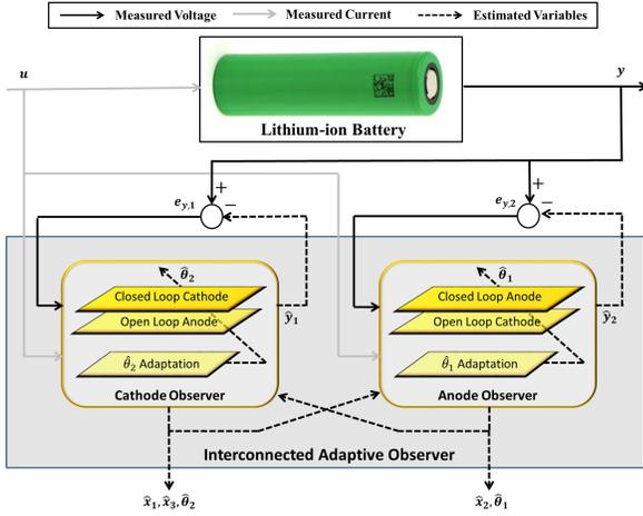
Fig. 2. Interconnected adaptive observer structure for the estimation of lithium concentration states ( $\hat{x}_1$  and  $\hat{x}_2$ ), total cell capacity ( $\hat{x}_3$ ), anode diffusion coefficient ( $\hat{\theta}_1$ ), and the SEI layer ionic conductivity ( $\hat{\theta}_2$ ).
