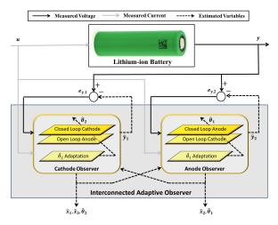
Fig. 2. Interconnected adaptive observer structure for the estimation of lithium concentration states  $(\hat{x}_1 \text{ and } \hat{x}_2)$ , total cell capacity  $(\hat{x}_3)$ , anode diffusion coefficient  $(\hat{\theta}_1)$ , and the SEI layer ionic conductivity  $(\hat{\theta}_2)$ .
