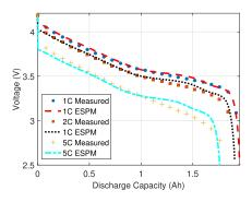
Fig. 12. Comparison of ESPM output voltage with measured cell voltage for 1C, 2C, and 5C constant current discharge cycles at 23 °C.
