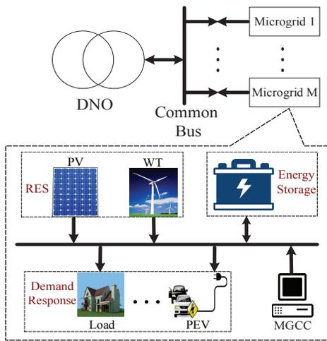
Fig. 1. Schematic of microgrid system considered in this work.
