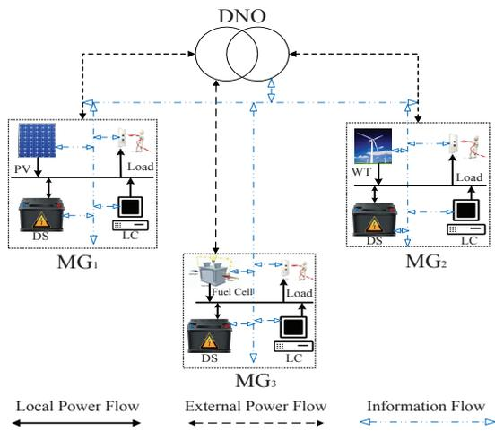
Fig. 3. Schematic of the studied microgrids.
