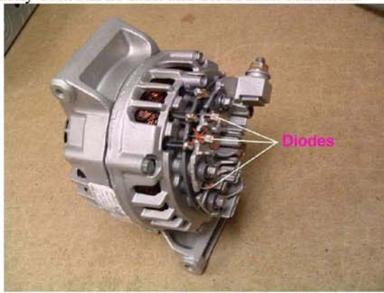
FIGURE 9. RECTIFIER FAULT SIMULATION.
