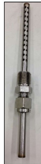
Figure 18 Designed diffuser to disperse O 2 into the exhaust stream
