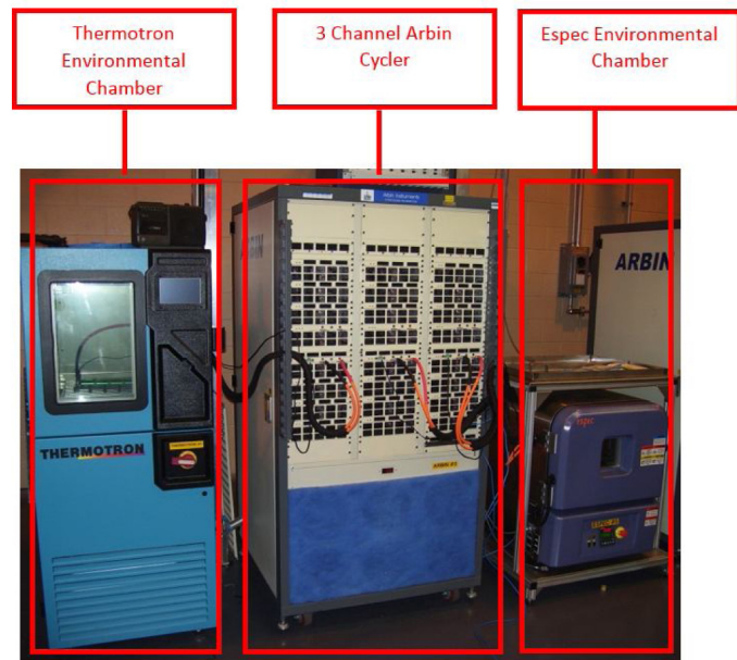
Figure 9. Arbin BT2000 Cycler along with Espec and Thermotron environmental chambers
