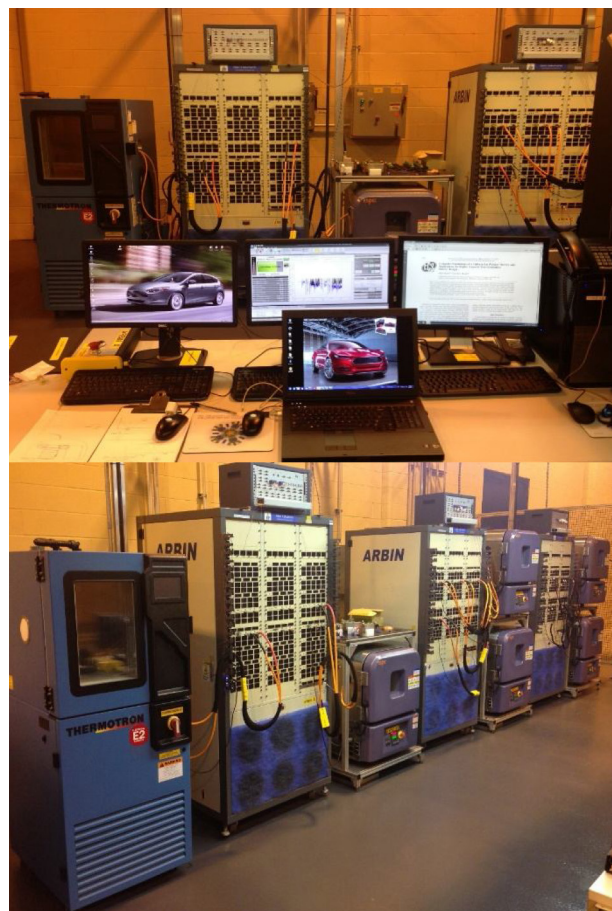
Figure 10. Experimental setup including cyclers, environmental chambers, and data acquisition systems.
