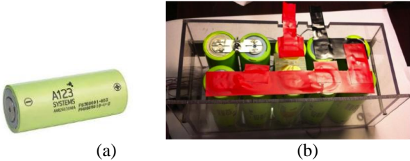
Fig 3. (a) A123 Lithium ion phosphate (LiFePO4) battery cell. Dimensions: diameter (D) =26mm, length (l) =65mm. (b) Battery module geometry, cell #1 is the one located in the top left while cell # 10 is the one located in the bottom right.
