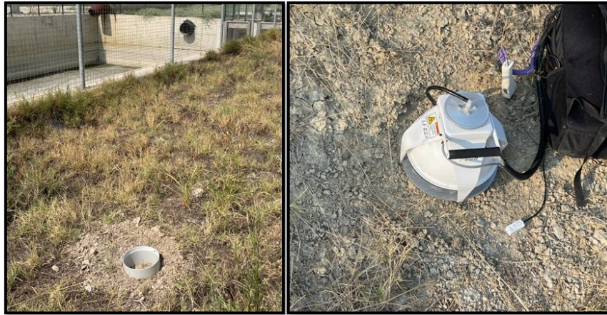
Figure 1: Soil collar installed into the ground for measurement (left), and soil flux measurement at Kızıldere (right).
