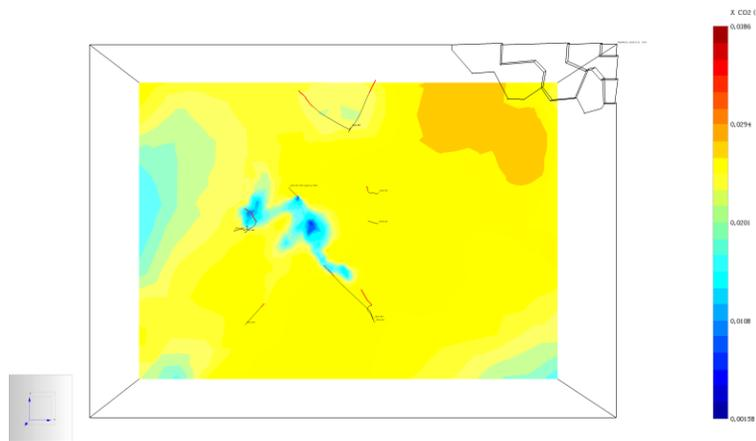
Figure 11 CO<sub>2</sub> Mass Fraction @Reservoir Depth (2200 BSL), 2 Years After CO<sub>2</sub> Injection
