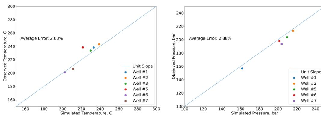
**Figure 4 Natural State Temperature and Pressure Matches at 9 5/8" depths**
