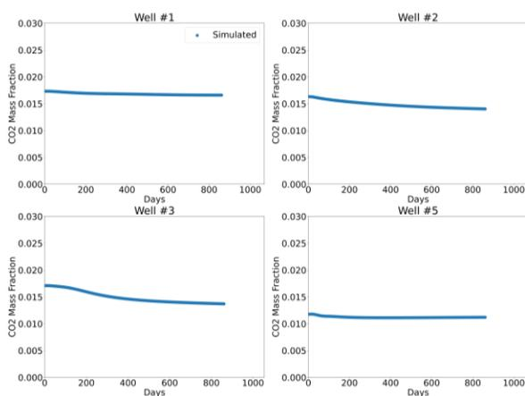
Figure 8 Carbon-Dioxide Mass Fractions of Production Wells after NCG injection
