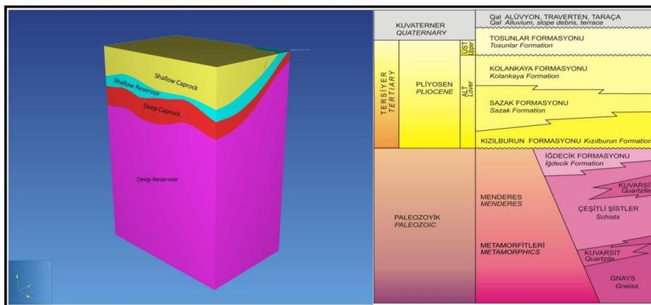
Figure 2 3D Conceptual Model of the Localized Model (left), General Stratigraphy of Kızıldere Field (right), (Şimşek et al, 2009)
