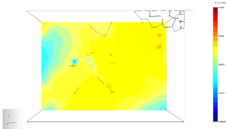
Figure 9 CO<sub>2</sub> Mass Fraction @Reservoir Depth (2200 BSL), Prior to Brine Injection.
