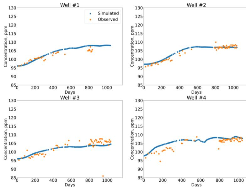
Figure 6 Calibration Results of Chloride Breakthrough Curves
