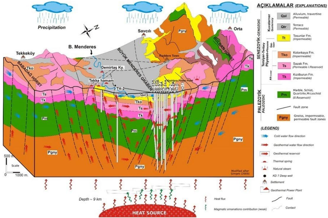
Figure 1 Conceptual Model of Kızıldere Field, (modified after Şimşek et al, 2009).
