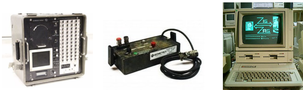
Figure 1: (Left) A photograph of a Nimbus Instruments Model ES-1210F like the one used to acquire the 1985 survey. (Credit: e-bay). (Centre) A photograph of an HVB-1 seismic trigger/timer like the one used in the 1985 survey (Photo credit: Geomatrix). (Right) A photograph of an Apple IIe like the one used to process the 1985 survey (Photo credit: Wikipedia).
